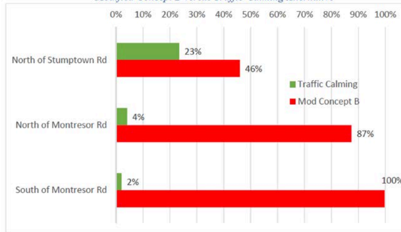
Figure 4: 2040 Southbound Morning Peak Period Traffic Growth from 2016: Modified Concept B versus Traffic-Calming Alternative
